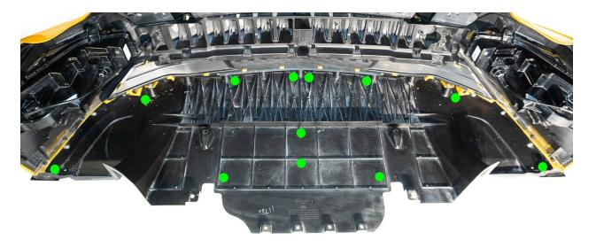
Each LVA front splitter comes with 12 sets of splitter hardware. We suggest repeating Step 6 for all of the "green-dot" locations shown above. We strongly urge our customers to place an emphasis on mounting a significant percentage of their mounting hardware as close to the "front-edge" of the bumper as possible.
