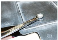
Place the "allen bolt" through the rounded "finishing-cup washer" and insert facing upwards going through the splitter with the threads sticking out of the belly-pan. Next, place the "flat washer" around the upward facing bolt, followed by threading the corresponding "nylon lock nut" onto the exposed bolt. Use your 11mm wrench to hold the "nylon lock nut" in place, while tightening the 5/32 allen bolt from the bottom. Reference photo below for a more detailed look:
