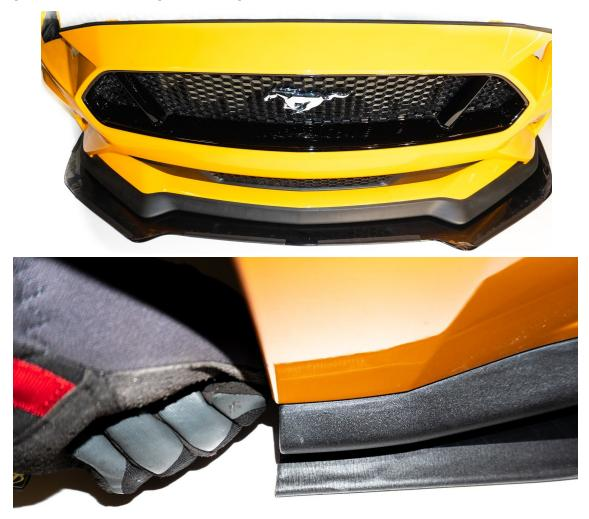
Align both ends of the bumper flush against the back of the splitter, as shown in the photo above.
