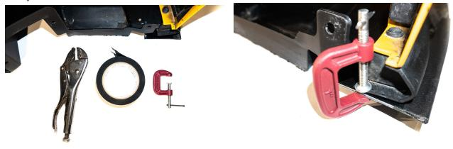
This can be done using a few different tools. We prefer the "C-Clamp" method (shown above). However, vice grips or good ol' tape will work as well. The goal is to hold the splitter in place during the upcoming drilling process. You may want to ask for assistance during this step.
