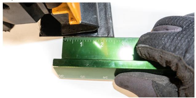
After aligning the bumper flush against the back of the splitter, measure both sides along the back most edge to center the bumper. The splitter should protrude the EXACT same amount on both the driver's and passenger's sides. You may want to ask for assistance during this process to minimize scratching on the splitter.
