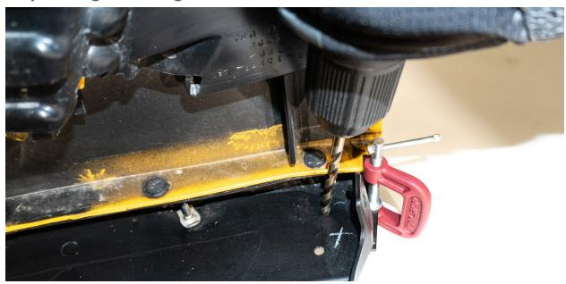
Utilizing the ¼ inch drill bit, drill through the factory belly-pan and LVA splitter. Start with one hole on each side located near your clamping device. These holes will ensure that the splitter stays in place throughout the rest of the installation.
