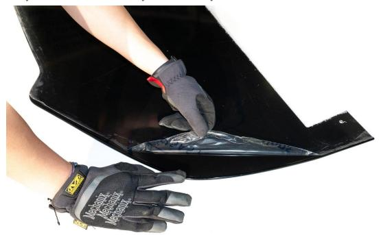
After drilling all 12 of your hardware holes through both the OEM belly-pan and front splitter, remove the bumper from the splitter. At this time, peel the protective film from BOTH sides of the splitter.
